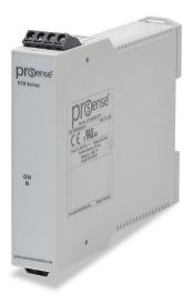
ProSense temperature transmitter, isolated, Pt100 RTD input, 0 to 500 deg F fixed, 4-20 mA output, 12-35 VDC operating voltage, 35mm DIN rail mount, removable screw terminal plugs.
