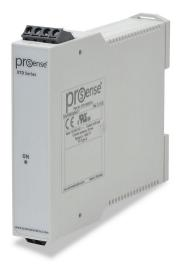
ProSense temperature transmitter, isolated, Type K thermocouple input, 0 to 500 deg F fixed, 4-20 mA output, 12 to 35 VDC operating voltage, 35mm DIN rail mount, removable screw terminal plugs.
