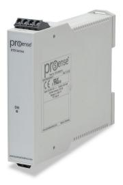
ProSense temperature transmitter, isolated, Type K thermocouple input, 0 to 500 deg F fixed, 4-20 mA output, 12-35 VDC operating voltage, 35mm DIN rail mount, removable screw terminal plugs.
