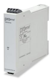
ProSense temperature transmitter, isolated, Type J thermocouple input, 0 to 500 deg F fixed, 4-20 mA output, 12-35 VDC operating voltage, 35mm DIN rail mount, removable screw terminal plugs.
