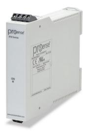
ProSense temperature transmitter, isolated, Pt100 RTD input, 0 to 300 deg F fixed, 4-20 mA output, 12 to 35 VDC operating voltage, 35mm DIN rail mount, removable screw terminal plugs.
