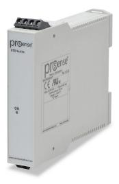
ProSense temperature transmitter, isolated, Type K thermocouple input, 0 to 300 deg F fixed, 4-20 mA output, 12-35 VDC operating voltage, 35mm DIN rail mount, removable screw terminal plugs.
