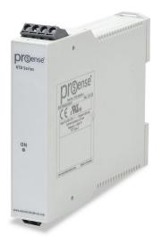
ProSense temperature transmitter, isolated, Type J thermocouple input, 0 to 300 deg F fixed, 4-20 mA output, 12-35 VDC operating voltage, 35mm DIN rail mount, removable screw terminal plugs.
