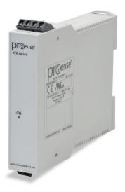
ProSense temperature transmitter, isolated, Type T thermocouple input, 0 to 200 deg F fixed, 4-20 mA output, 12-35 VDC operating voltage, 35mm DIN rail mount, removable screw terminal plugs.
