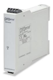
ProSense temperature transmitter, isolated, Pt100 RTD input, 0 to 200 deg F fixed, 4-20 mA output, 12-35 VDC operating voltage, 35mm DIN rail mount, removable screw terminal plugs.
