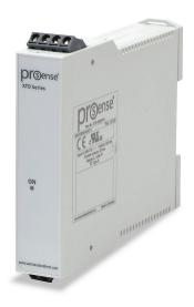
ProSense temperature transmitter, isolated, Type K thermocouple input, 0 to 200 deg F fixed, 4-20 mA output, 12-35 VDC operating voltage, 35mm DIN rail mount, removable screw terminal plugs.
