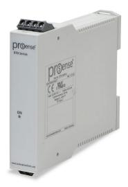
ProSense temperature transmitter, isolated, Type J thermocouple input, 0 to 200 deg F fixed, 4-20 mA output, 12-35 VDC operating voltage, 35mm DIN rail mount, removable screw terminal plugs.
