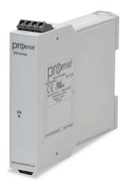
ProSense temperature transmitter, isolated, Type J thermocouple input, 0 to 200 deg F fixed, 4-20 mA output, 12 to 35 VDC operating voltage, 35mm DIN rail mount, removable screw terminal plugs.
