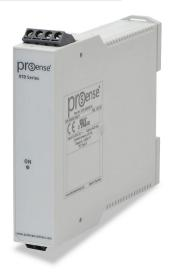
ProSense temperature transmitter, isolated, Type K thermocouple input, 0 to 2000 deg F fixed, 4-20 mA output, 12 to 35 VDC operating voltage, 35mm DIN rail mount, removable screw terminal plugs.
