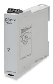
ProSense temperature transmitter, isolated, Type K thermocouple input, 0 to 2000 deg F fixed, 4-20 mA output, 12-35 VDC operating voltage, 35mm DIN rail mount, removable screw terminal plugs.
