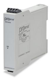
ProSense temperature transmitter, isolated, Type K thermocouple input, 0 to 1500 deg F fixed, 4-20 mA output, 12-35 VDC operating voltage, 35mm DIN rail mount, removable screw terminal plugs.
