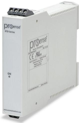
ProSense temperature transmitter, isolated, Pt100 RTD input, 0 to 100 deg F fixed, 4-20 mA output, 12-35 VDC operating voltage, 35mm DIN rail mount, removable screw terminal plugs.
