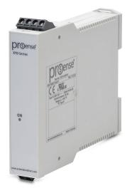
ProSense temperature transmitter, isolated, Type K thermocouple input, 0 to 100 deg F fixed, 4-20 mA output, 12-35 VDC operating voltage, 35mm DIN rail mount, removable screw terminal plugs.
