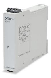
ProSense temperature transmitter, isolated, Type J thermocouple input, 0 to 100 deg F fixed, 4-20 mA output, 12 to 35 VDC operating voltage, 35mm DIN rail mount, removable screw terminal plugs.
