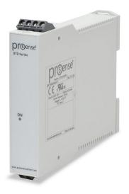
ProSense temperature transmitter, isolated, Type J thermocouple input, 0 to 100 deg F fixed, 4-20 mA output, 12-35 VDC operating voltage, 35mm DIN rail mount, removable screw terminal plugs.
