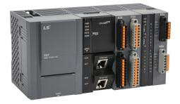
LS Electric XMC programmable motion controller, microSD card slot, Ethernet and USB B ports, EtherCAT Master and Modbus TCP, up to (16) axes and up to (18) virtual axes, external 24 VDC required. Optional XEL-BSSCT bus coupler for I/O expansion with XGB modules.
