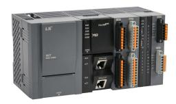
LS Electric XMC programmable motion controller, microSD card slot, Ethernet and USB B ports, EtherCAT Master and Modbus TCP, up to (8) axes and up to (9) virtual axes, external 100-240 VAC required. Optional XEL-BSSCT bus coupler for I/O expansion with XGB modules.
