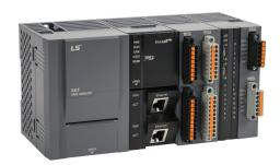
LS Electric XMC programmable motion controller, microSD card slot, Ethernet and USB B ports, EtherCAT Master and Modbus TCP, up to (8) axes and up to (9) virtual axes, external 24 VDC required. Optional XEL-BSSCT bus coupler for I/O expansion with XGB modules.
