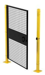
Velox machine guarding door, left hinged, swing out, 48 x 72in, 2 x 2in grid, carbon steel, yellow and black. 2 door posts XG5506D and mounting hardware included.
