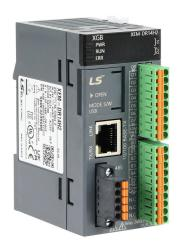
LS Electric XGB PLC, 24 VDC required, Ethernet, serial and USB B ports, Discrete Input: 8-point, DC, Discrete Output: 6-point, relay, 4 high-speed input point(s).
