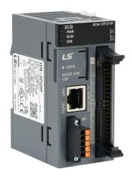
LS Electric XGB PLC, 24 VDC required, Ethernet, serial and USB B ports, Discrete Input: 16-point, DC, Discrete Output: 16-point, sourcing, 4 high-speed input point(s), 6 high-speed output point(s). Requires XTB-40H terminal block and C40HH-xxSB-XBI cable.
