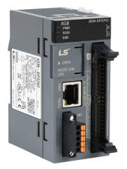
LS Electric XGB PLC, 24 VDC required, Ethernet, serial and USB B ports, Discrete Input: 16-point, DC, Discrete Output: 16-point, sourcing, 4 high-speed input point(s), 2 high-speed output point(s). Requires XTB-40H terminal block and C40HH-xxSB-XBI cable.
