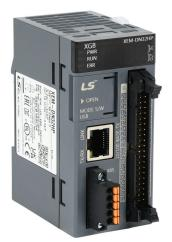
LS Electric XGB PLC, 24 VDC required, Ethernet, serial and USB B ports, Discrete Input: 16-point, DC, Discrete Output: 16-point, sinking, 4 high-speed input point(s), 6 high-speed output point(s). Requires XTB-40H terminal block and C40HH-xxSB-XBI cable.
