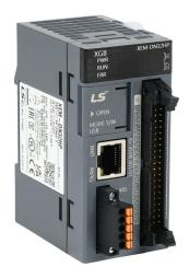
LS Electric XGB PLC, 24 VDC required, Ethernet, serial and USB B ports, Discrete Input: 16-point, DC, Discrete Output: 16-point, sinking, 4 high-speed input point(s), 12 high-speed output point(s). Requires XTB-40H terminal block and C40HH-xxSB-XBI cable.
