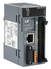
LS Electric XGB PLC, 24 VDC required, Ethernet, serial and USB B ports, Discrete Input: 16-point, DC, Discrete Output: 16-point, sinking, 4 high-speed input point(s), 2 high-speed output point(s). Requires XTB-40H terminal block and C40HH-xxSB-XBI cable.
