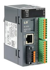
LS Electric XGB PLC, 24 VDC required, Ethernet, serial and USB B ports, Discrete Input: 8-point, DC, Discrete Output: 8-point, sinking, 4 high-speed input point(s), 2 high-speed output point(s).
