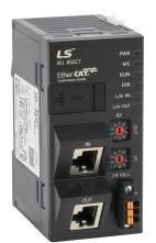
LS Electric XGB bus coupler, 24 VDC, (2) Ethernet (RJ45) and (1) USB B port(s), EtherCAT Slave, 100 Mbps. For use with LS Electric XGB series I/O modules.
