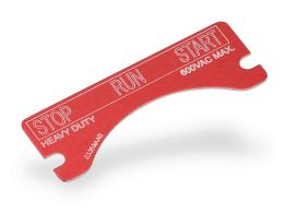
Killark legend plate, aluminum, rectangular, red background, white engraved text, legend plate marking "STOP RUN START". For use with FXCS and XCS series control stations. Mounting screws included.
