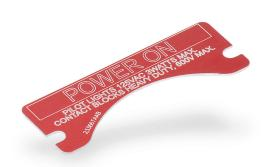
Killark legend plate, aluminum, rectangular, red background, white engraved text, legend plate marking "POWER ON". For use with FXCS and XCS series control stations. Mounting screws included.
