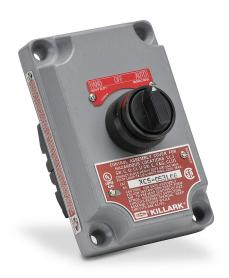
Killark control station cover assembly, hazardous location rated, single selector switch, knob, 3-position, black, spring return to center from right, maintained center and left, (2) N.O. contact(s), legend plate marking "HAND OFF AUTO".
