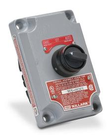
Killark control station cover assembly, hazardous location rated, single selector switch, knob, 3-position, black, maintained, (2) N.O./(2) N.C. contact(s), legend plate marking "HAND OFF AUTO".
