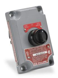
Killark control station cover assembly, hazardous location rated, single selector switch, knob, 3-position, black, maintained, (1) N.O./(1) N.C. contact(s), legend plate marking "HAND OFF AUTO".
