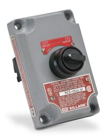
Killark control station cover assembly, hazardous location rated, single selector switch, knob, 2-position, black, spring return from right, (1) N.O./(1) N.C. contact(s), legend plate marking "OFF ON".
