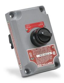
Killark control station cover assembly, hazardous location rated, single selector switch, knob, 2-position, black, spring return from right, (1) N.O./(1) N.C. contact(s), legend plate marking "OFF ON".
