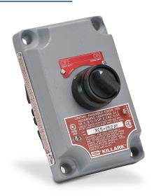
Killark control station cover assembly, hazardous location rated, single selector switch, knob, 2-position, black, maintained, (2) N.O./(2) N.C. contact(s), legend plate marking "OFF ON".
