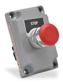
Killark control station cover assembly, hazardous location rated, single pushbutton, mushroom, red, push-pull, (1) N.O./(1) N.C. contact(s), (3) two-sided legend plate(s), legend plate marking "START,STOP / EMERGENCY STOP, RESET / blank, RESET".
