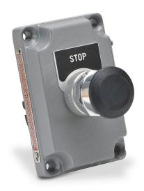
Killark control station cover assembly, hazardous location rated, single pushbutton, mushroom, black, push-pull, (1) N.O./(1) N.C. contact(s), (3) two-sided legend plate(s), legend plate marking "START,STOP / EMERGENCY STOP, RESET / blank, RESET".
