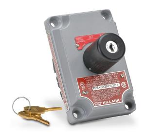
Killark control station cover assembly, hazardous location rated, single selector switch, key-operated, 3-position, black, spring return to center from left, maintained center and right, (2) N.O. contact(s), legend plate marking "HAND OFF AUTO".
