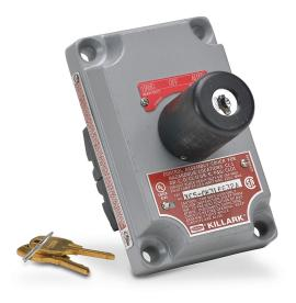
Killark control station cover assembly, hazardous location rated, single selector switch, key-operated, 3-position, black, spring return to center from right, maintained center and left, (2) N.O. contact(s), legend plate marking "HAND OFF AUTO".
