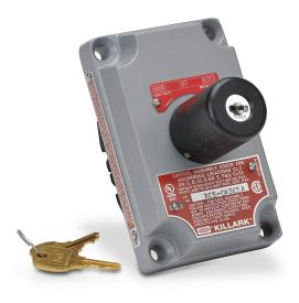
Killark control station cover assembly, hazardous location rated, single selector switch, key-operated, 3-position, black, maintained, (2) N.O./(2) N.C. contact(s), legend plate marking "HAND OFF AUTO".
