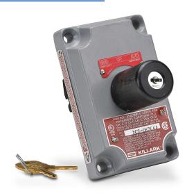
Killark control station cover assembly, hazardous location rated, single selector switch, key-operated, 3-position, black, maintained, (1) N.O./(1) N.C. contact(s), legend plate marking "HAND OFF AUTO".
