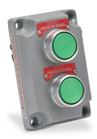
Killark control station cover assembly, hazardous location rated, two pushbuttons, green/green, momentary, (1) N.O. and (1) N.O. contact(s), legend plate marking "START / START".
