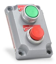
Killark control station cover assembly, hazardous location rated, two pushbuttons, red/green, momentary, (1) N.O. and (1) N.C. contact(s), legend plate marking "START / STOP".
