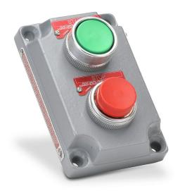
Killark control station cover assembly, hazardous location rated, two pushbuttons, red/green, momentary, (1) N.O/(1) N.C. and (1) N.O/(1) N.C. contact(s), legend plate marking "START / STOP".
