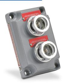
Killark control station cover assembly, hazardous location rated, two pilot lights, indicating light, clear/clear, 110 VAC/VDC LED, clear/white, operator only, (2) blank legend plate(s).
