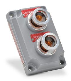
Killark control station cover assembly, hazardous location rated, two pilot lights, indicating light, amber/amber, 110 VAC/VDC LED, amber, operator only, (2) blank legend plate(s).
