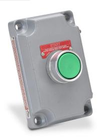
Killark control station cover assembly, hazardous location rated, single pushbutton, green, momentary, (1) N.O. contact(s), legend plate marking "START".
