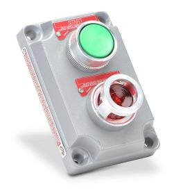
Killark control station cover assembly, hazardous location rated, single pilot light, single pushbutton, green, 110 VAC/VDC LED, red, momentary, (1) N.O. contact(s), blank legend plate(s), legend plate marking "START".
