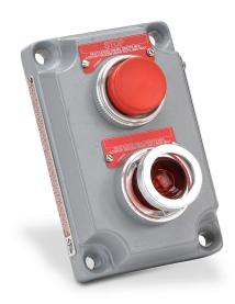
Killark control station cover assembly, hazardous location rated, single pilot light, single pushbutton, red, 110 VAC/VDC LED, red, momentary, (1) N.C. contact(s), blank legend plate(s), legend plate marking "STOP".
