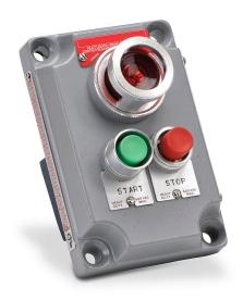
Killark control station cover assembly, hazardous location rated, single pilot light, two mini-pushbuttons, red/green, 110 VAC/VDC LED, red, momentary, (1) N.O./(1) N.C. contact(s), blank legend plate(s), legend plate marking "START, STOP".
