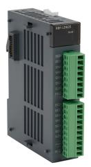
LS Electric XGB load cell input module, 2-channel, voltage, 15-bit resolution, input voltage signal range(s) of 0-6 mV/VDC. For use with 5 VDC four- or six-wire load cells. Removable terminal blocks included.
