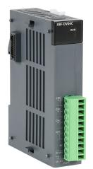
LS Electric XGB analog output module, 4-channel, voltage, 14-bit, output voltage signal range(s) of 0-5 VDC, 1-5 VDC, 0-10 VDC and +/- 10 VDC, external 24 VDC required.
