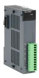
LS Electric XGB analog output module, 4-channel, voltage, 14-bit, output voltage signal range(s) of 0-5 VDC, 1-5 VDC, 0-10 VDC and +/- 10 VDC, external 24 VDC required.
